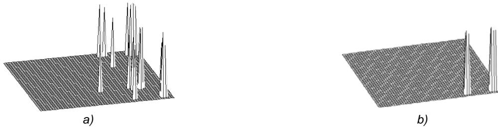
Fig. 3. Comparison between 'classical' and no-reference DTT algorithms in the inspection of a 2-mm thick CFRP sample:
